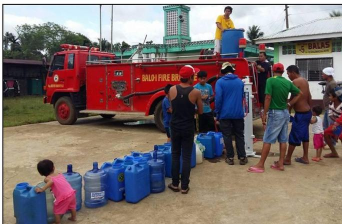
*The photo shows an old fire engine that has been used to transport raw water, and, with the addition of a SkyHydrant treat the water, making it safe to drink before its distribution.*
